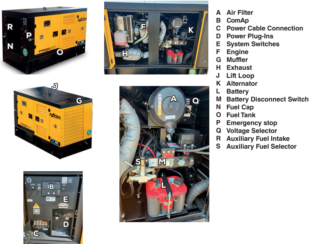
FIG. 1 MACHINE & TANK COMPONENTS (TYPICAL)
