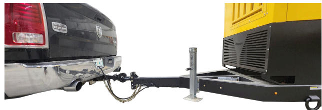
Jack Rotated/Handle Secured
