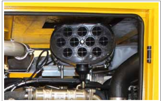
FIG. 33 AIR CLEANER (TYPICAL)
