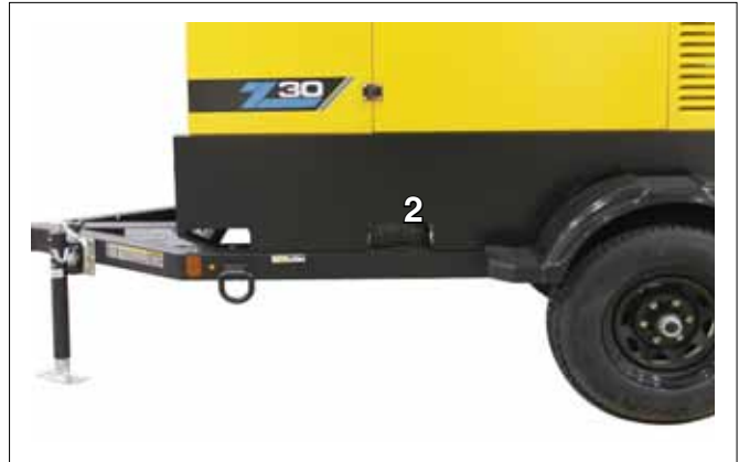
FIG. 10 FORKLIFT POCKETS (TYPICAL)
